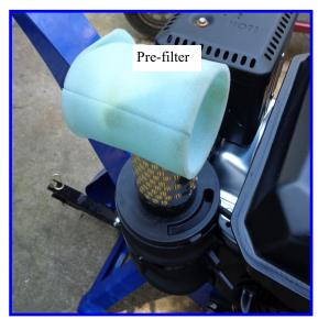
Honda engines have a different filter, consult your engine manual for directions on cleaning.
