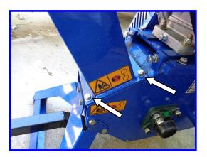
• If the starter is hard to pull make sure the blade is not jammed. If you pull a starter cord with the blade jammed you will break the rope.
