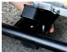
2. Fasten the nut to the bolt, tighten with a wrench.
