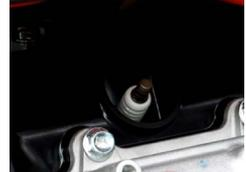
2. Use a ratchet and 13/16 spark plug socket (included with your generator) to unscrew and remove the spark plug.
