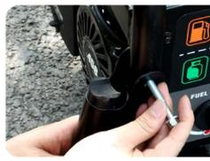
2. Fasten the nut to the bolt and tight with a wrench.
