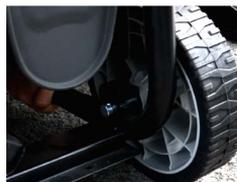
2. Insert the R pin into the hole at the end of the wheel shaft to prevent the wheel from coming off.
