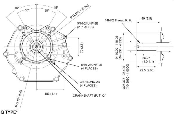
P.D.165.1(6.50) 45° 45° 30° 30° 88.5 (3.48) 7/16 - 20UNF - 2B 5/16-24UNF-2B 56 (2.2) (2 PLACES) 6.30 - 6.35 0 (0.248 - 0.250) Ф110.00 - 110.05 (Ф4.331 - 4.333) 70 (2.8) (**b**) 28 (1.1) 21.69 - 21.82 (0.854 - 0.859) 5/16-24UNF-2B Ф25.375 - 25.400 (Ф0.9990 - 1.0000) 72.2 (2.84) (4 PLACES) 3/8-16UNC-2B (4 PLACES)
